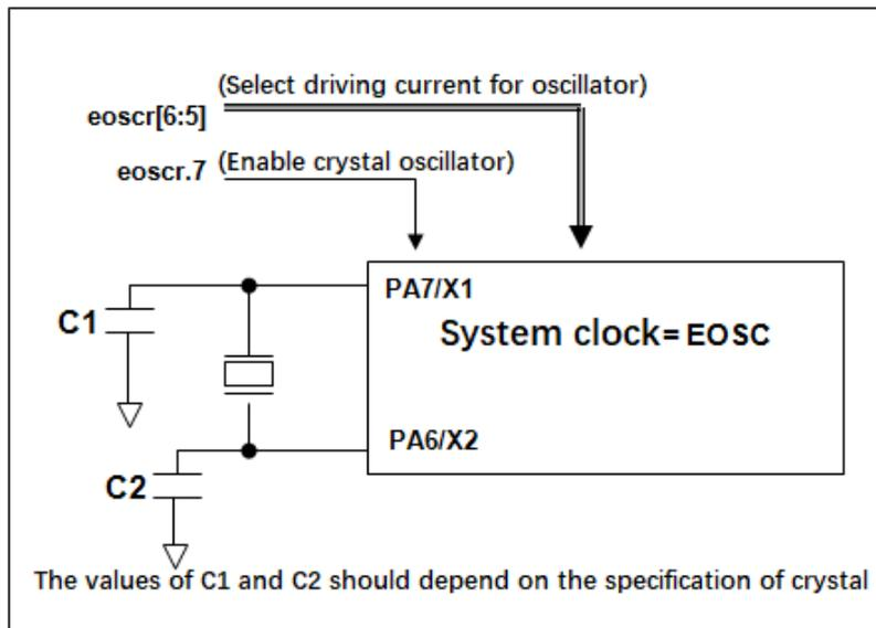
The capacitor values of C1 and C2 shall be adjusted to:
